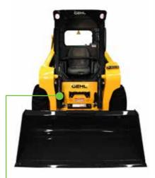
DETWEEN-THE-TIRE design keeps machine length short and compact. On the R190
